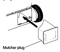
**ACAUTION:** Do not run your lawn mower without mulcher plug in place or approved clipping deflector or grass catcher in place. Never attempt to operate the lawn mower with the rear door removed or propped open.
